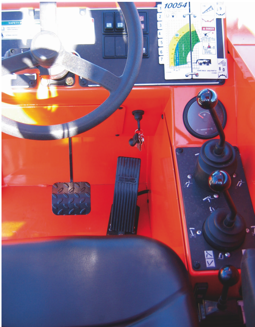
Showcase operators who preferred dual controls found they were easier to handle. Only three machines in the Showcase had dual joysticks.
