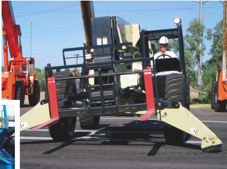
(Above) Ingersoll Rand's unique frame-mounted stabilizers aren't designed to support the entire weight of the machine and load, but they allow frame-sway to function when they're deployed.
