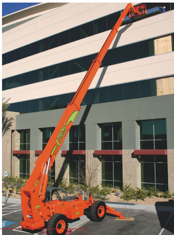
Xtreme XRM1267 lifts 3,000 pounds to a maximum reach of 53 feet 9 inches.
