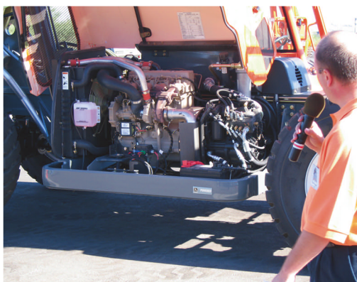
JLG's Dave Baxter points out the advantages of the side-mounted engine. Four of the 12 Showcase telehandlers had engines in pods mounted on the side of the frame.
