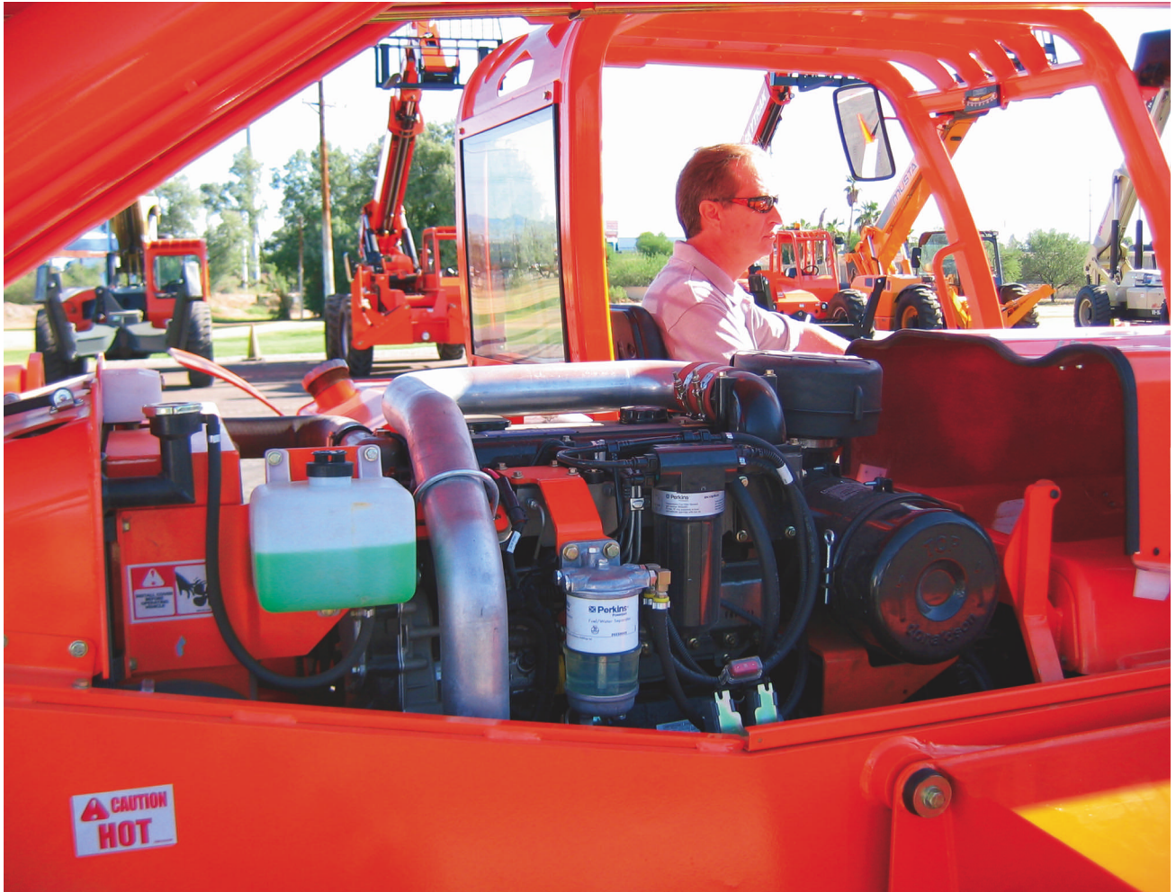
Xtreme is a great example of a well-thought-out, mid-engine installation. Five Showcased machines carried their engines mounted nearly centered within the frame.
