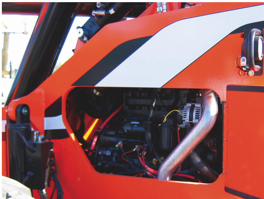
SkyTrak's rear-mounted in-frame engine. Three of the 12 telehandlers reviewed at the Showcase had engines mounted in-frame, near the rear of the machine.
