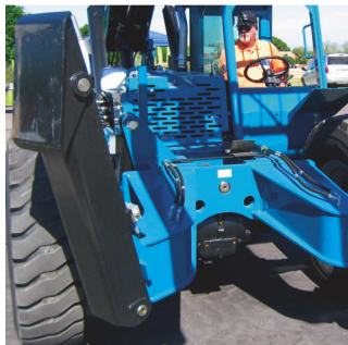
(Above) Ingersoll Rand's unique frame-mounted stabilizers aren't designed to support the entire weight of the machine and load, but they allow frame-sway to function when they're deployed.
