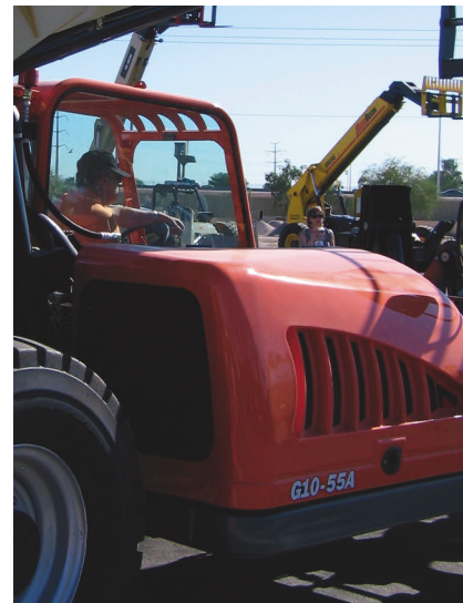
The center spine impacts the engine position and allows for better line of sight.
